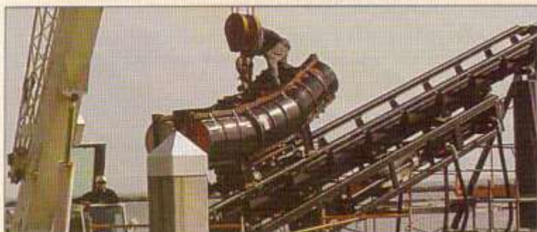
The crane crew resets the "Flying Pig" test vehicle during factory testing on San Francisco Bay. The six 55-gallon drums are weighted with concrete to match the final themed vehicle.
