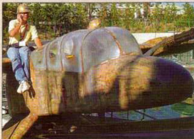
Marcial Godoy of Birket Engineering, Inc. adjusts the RF pyrotechnic system inside the themed prop seaplane while it rests on its launcher backstage. Among the challenges of creating control systems for entertainment is hiding or disguising them in unusual places while preserving easy access.
